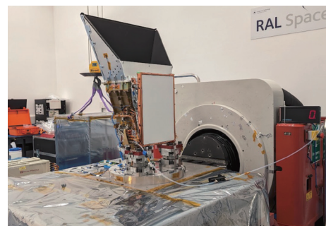
Fig. 5 SXI Telescope PFM during vibration test conducted at RAL Space (credit to S. Sembay, U. Leicester, UK)
